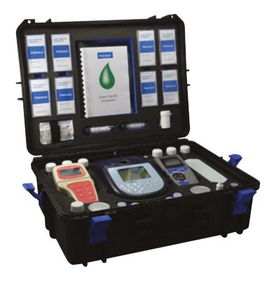
Designed to aid operational monitoring, the kit can also be customised by selecting from other 100 additional Palintest® parameters for use with the Photometer 7500.
