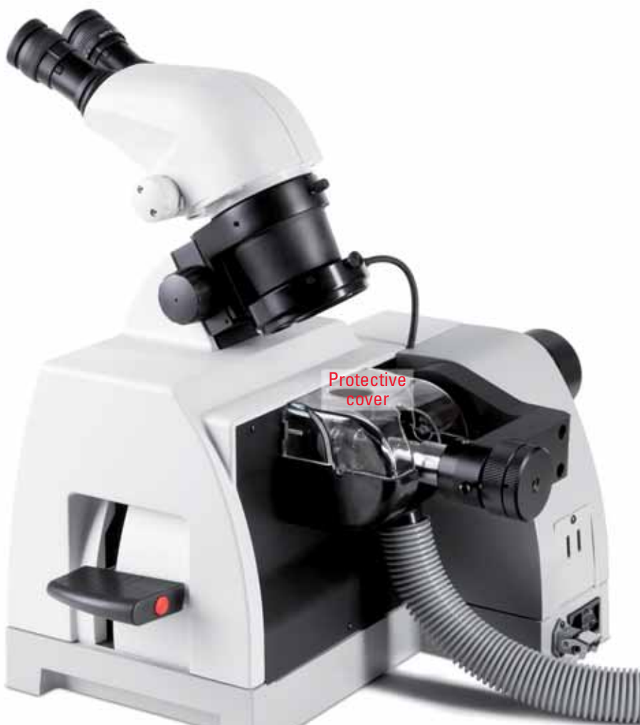
Exhaust tube connection to the extraction and filtration unit
