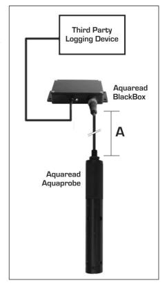
For applications where water quality data needs to be collected remotely, the BlackBox is again the answer. In this configuration, logging device is replaced by a third party telemetry device that can transmit data to a remote monitoring station anywhere in the world.
