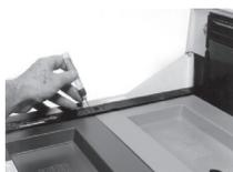
**Figure 30: Lubricating The Main Frame**
