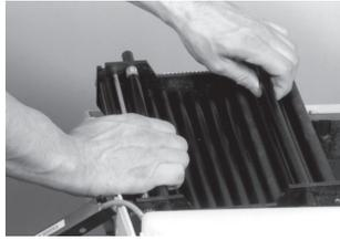
Figure 25: Removing the Developer Transport Module
