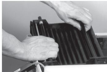
Figure 14: Removing Developer Transport Module
