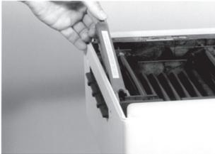
Figure 24: Removing the Film Sensor Bar Assembly
