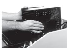
**Figure 33: Lifting out Washer/Dryer Module**
