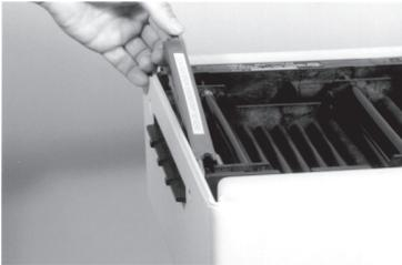
Figure 13: Lifting up Film Sensor Bar
