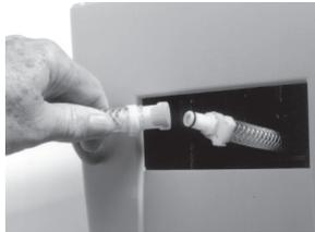
**Figure 11: Connecting Hose from water inlet solenoid**
