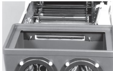
Figure 16: Attaching Loader, mounting bracket and wing nuts
