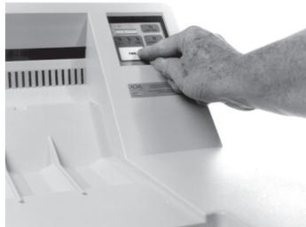
Figure 20: Depressing TIME Button (810 Basic shown)
