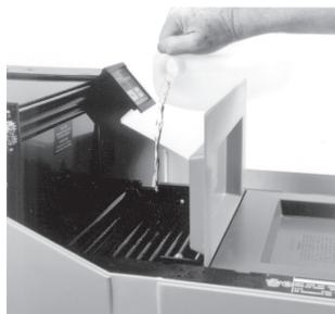
**Figure 18:** Loading Fixer Solution (Note the protective baffle by using the fixer evaporator cover between solution trays when pouring fixer. Use the same procedure with the cover for developer when pouring the developer).
