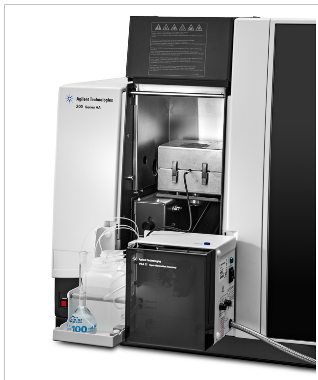
Figure 2. The ETC 60 electrothermal temperature controller (metal box in burner compartment) is an optional accessory for use with the VGA 77.
