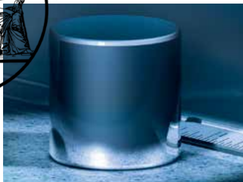
International Prototype Kilogram (IPK) at BIPM, a cylinder made of 90% platinum and 10% iridium.
