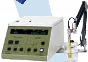
Model F-80 (benchtop) The world's first instrument capable of measuring pH at 0.001 resolution includes an integral computer with automatic calibration and a self-diagnostic function.
