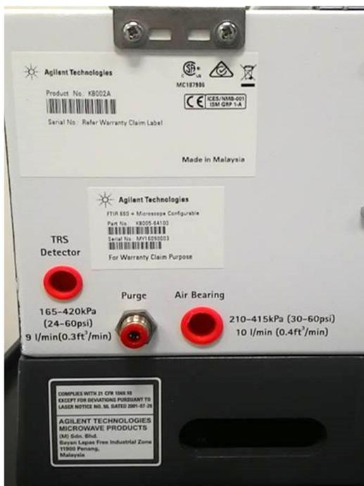
**Figure 1.** Laser safety label locations on the rear of the Agilent Cary 600 Series FTIR spectrometer
