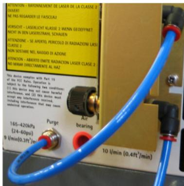
**Figure 6.** Purge fittings on the rear of the spectrometer
