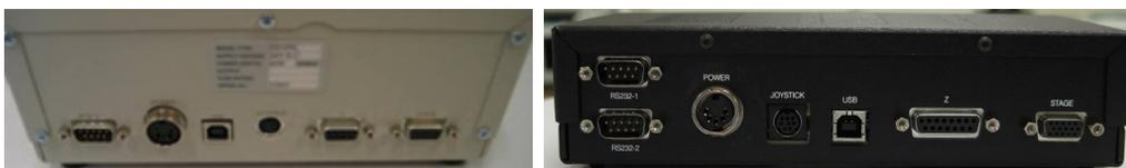
**Figure 12.** Older (left) and newer model (right) motorized stage controller connections
