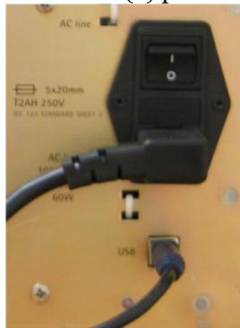
**Figure 8.** Power switch and socket on the rear of the microscope. USB to PC cable also shown.
