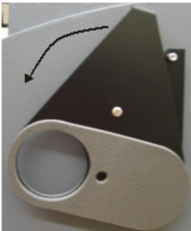
**Figure 16.** Side view of closed shutter and handle
