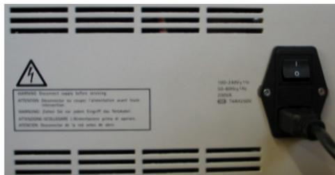
**Figure 5.** Power switch and socket on the rear of the spectrometer
