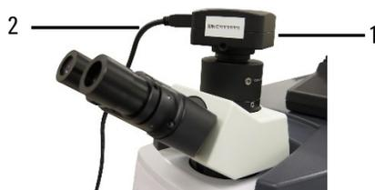
**Figure 11.** ToupCam camera and USB 3 cable
